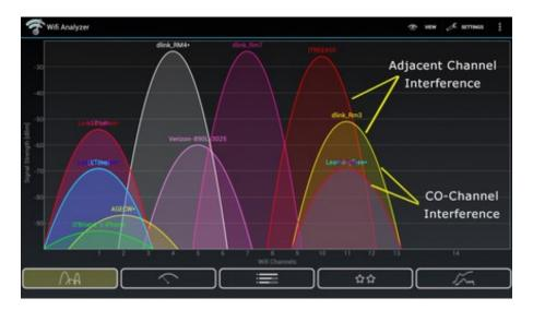
The Wi-Fi Analyzer tool provides an overview of the signals within the area. For the best performance, select Wi-Fi channels for AXIS where there are the least overlapping signals. Using the diagram as a reference, that would be channels 5 to 10.
